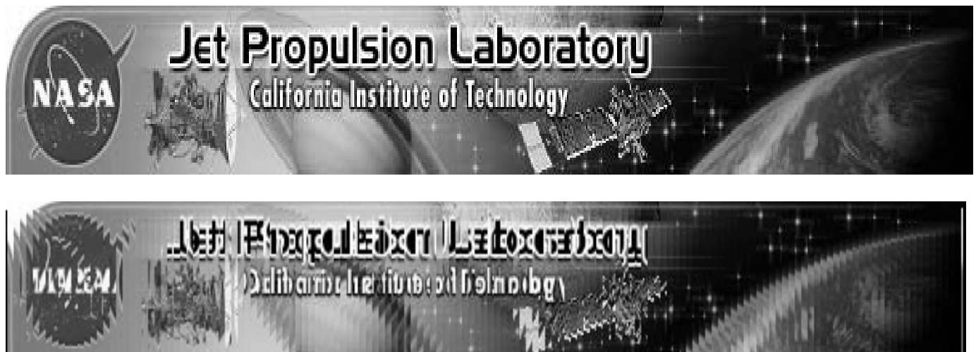
Figure 3: The Original Image (top) and the Effect of a Single-bit Fault in One of the Link Layer Registers (bottom).
